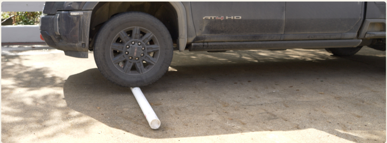
A loaded Sawgrass tube under the front tire of a three-quarter-ton pickup. The rods came out intact.
